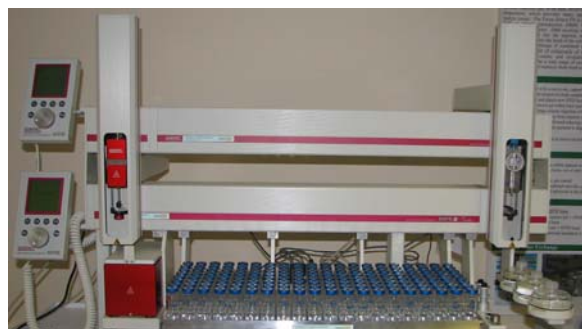
Figure 1: A dual-rail MPS 2 configured with a 2.5mL heated headspace syringe and a 25µL liquid syringe for the standard addition.
